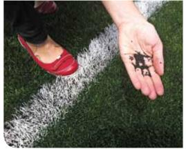
To provide shock absorbency, rubber granules are commonly used in synthetic grass, as seen here at an artificial sports field in Northbridge, NSW.
